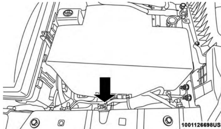
Auxiliary Switch Connections – Under Hood
