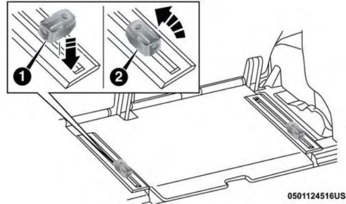
Installing Adjustable Slides
