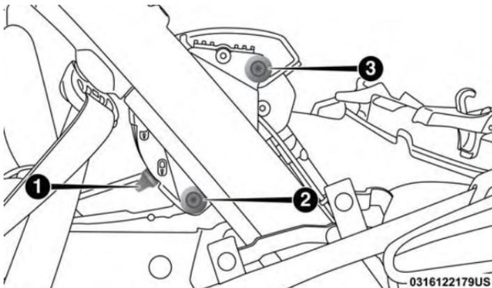
Lift Assist Mechanism In Place
