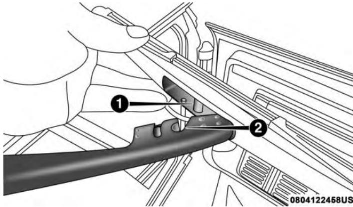
**Wiper Blade Removed From Wiper Arm**
