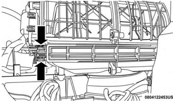
**Air Filter Retaining Tabs**
