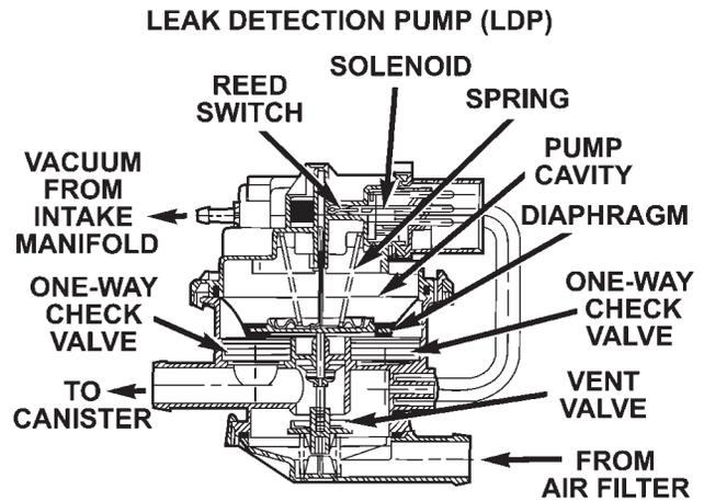
the PCM. This allows the PCM to monitor LDP pumping action as it turns the LDP solenoid on and off.
