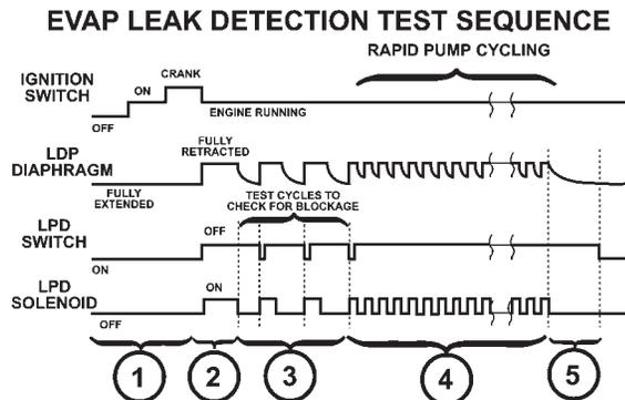
SECTION 1-P1495 LEAK DETECTION PUMP SOLENOID CIRCUIT CAN SET (KEY "ON")
