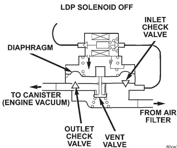
The pumping cycle is repeated as the solenoid is turned on and off. When the evaporative system begins to pressurize, the pressure on the bottom of
