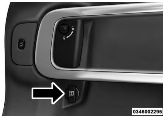
Rear Power Outlet
