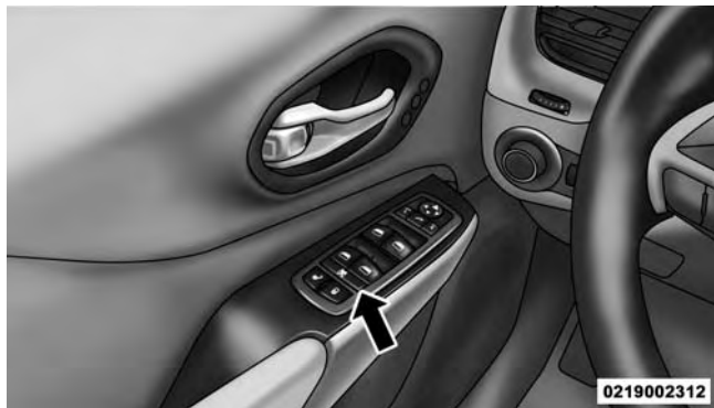
Window Lockout Switch
