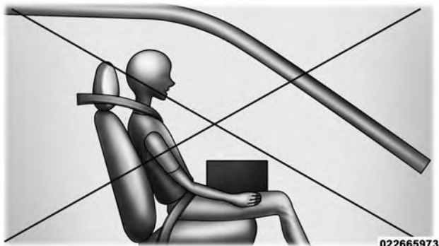
Not Seated Properly
